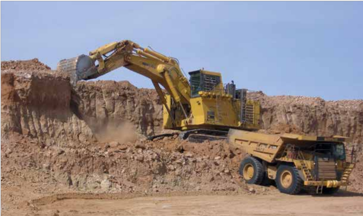
Fig. 5.1.8: Mining of unconsolidated Namakwa ore sands using front-end loaders (load-and-carry operation). The hardened layers are mined using hydraulic excavators in a backhoe configuration or by trackdozer. The mined material is transported by trucks to the mineral sizers where primary reduction takes place (Photo DERA).
