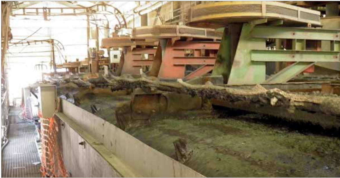
Fig. 5.3.5: Flotation of stibnite ore in the processing plant at Athens shaft (Photo DERA).
