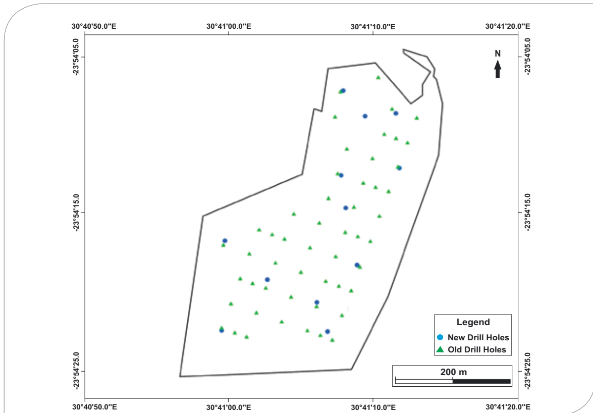
Fig. 5.3.11: Collar positions for 1984/1985 (old drill holes) and February 2010 (new drill holes) drilling campaigns on the OSD (modified after KING 2010).
