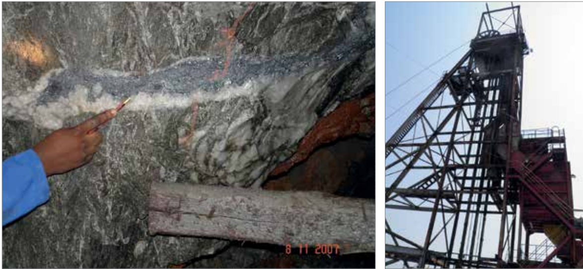
Fig. 5.3.4: Left: Primary mineralization of stibnite within a quartz-carbonate vein in the Athens shaft (920 m below ground; photo BGR). Right: head gear of the Athens shaft (Photo DERA).
