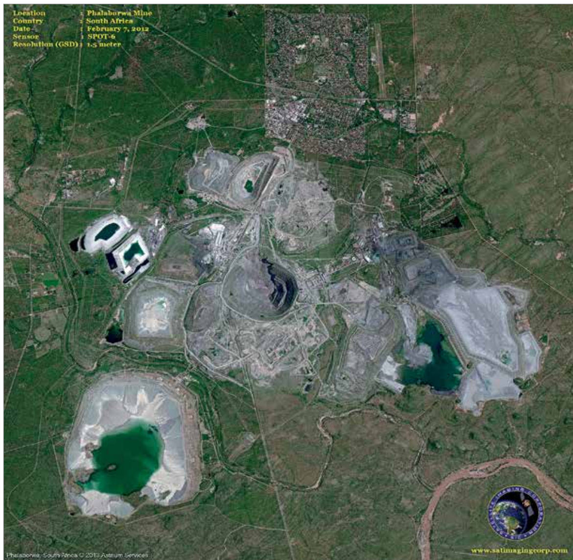
Fig. 5.2.19: Satellite image of the Phalaborwa mining operations with the four open pits (northern: Foskor open pit, VOD open pit, central: Palabora open pit (inactive), southern: P.P. & V. open pit), the processing plants and the tailings dams (Photo courtesy of SATELLITE IMAGING CORPORATION).
