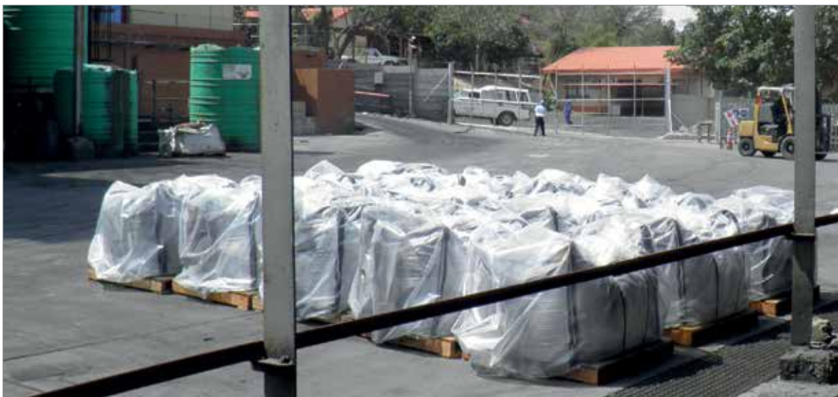
Fig. 5.3.6: Stibnite concentrate packed in 1 metric ton big packs for export (Photo DERA).
