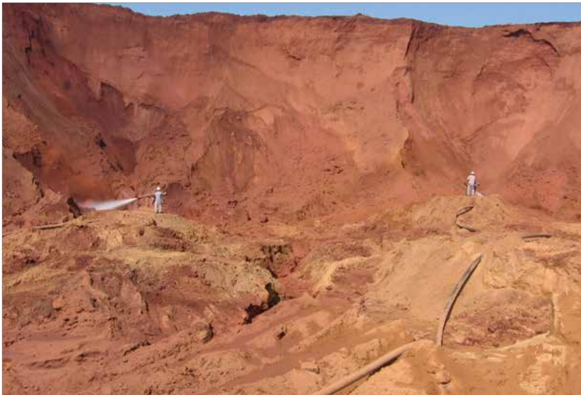
Fig. 5.1.13: Hydraulic mining of HM-rich sands at KZN Sands in KwaZulu-Natal, Republic of South Africa (Photo DERA).
