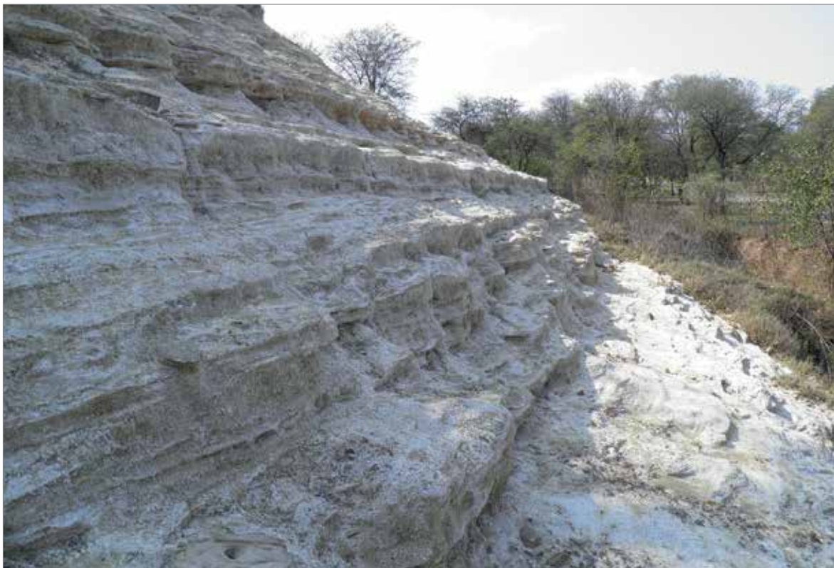
Fig. 5.3.10: Fine-grained, sandy to silty material of the new slimes dam (NSD; photo DERA).
