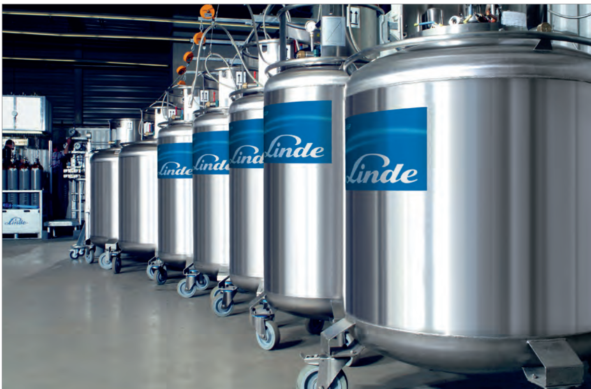
Fig. 29: Transport containers filled with 450 litres of liquid helium at Linde AG's Unterschleißheim factory, photo: Linde AG (with kind permission).
