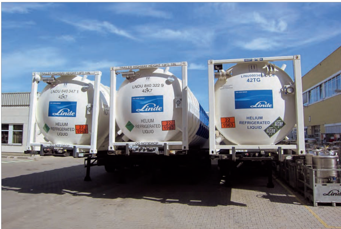
Fig. 27: ISO refrigerated container for transporting liquid helium at Linde AG's Unterschleißheim factory. The two containers at the left were produced by Linde Engineering, the container on the right by Gardner Cryogenics, Inc., photo: BGR.
