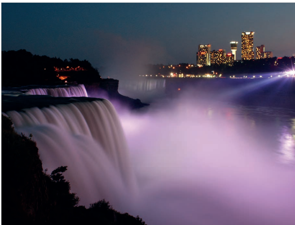
Fig. 18: At night, 4000 watt high-pressure xenon Osram floodlights illuminate the Niagara Falls between Canada and the USA. At a voltage of 21 volts they together produce a light intensity of 8 billion candela, photo: Ruben Yie/Wikipedia.
