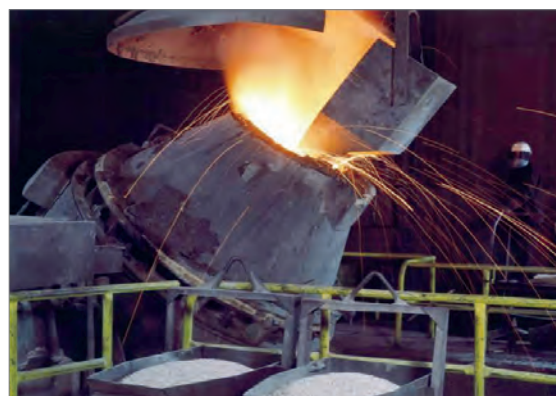
Fig. 16: Refining of a CrMoWVNbN stainless steel alloy in an argon-oxygen decarburisation vessel, photo: Goodwin Steel Castings/Wikipedia.
