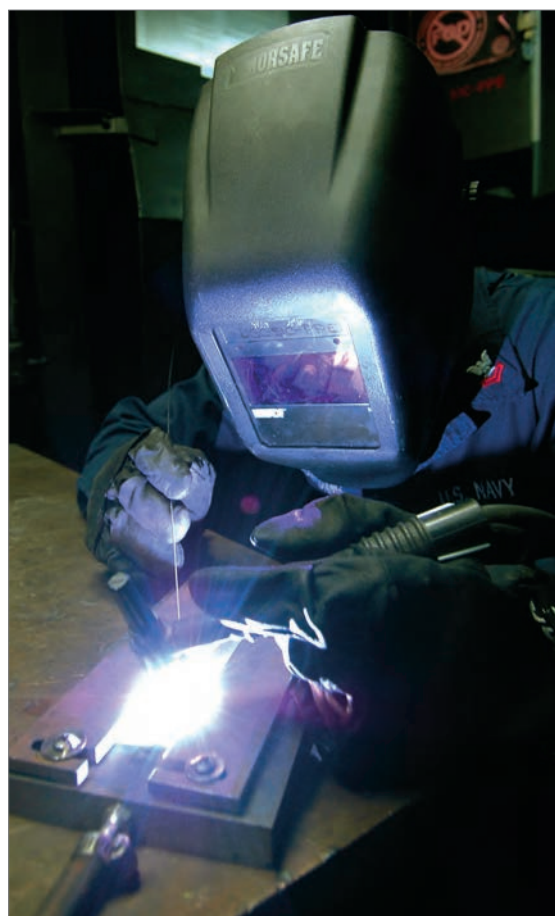
Fig. 9: Tungsten inert gas welding in an inert gas atmosphere of argon or helium is suitable for welding all metals and alloys where quality is more important than welding speed, photo: US Navy/Wikipedia.
