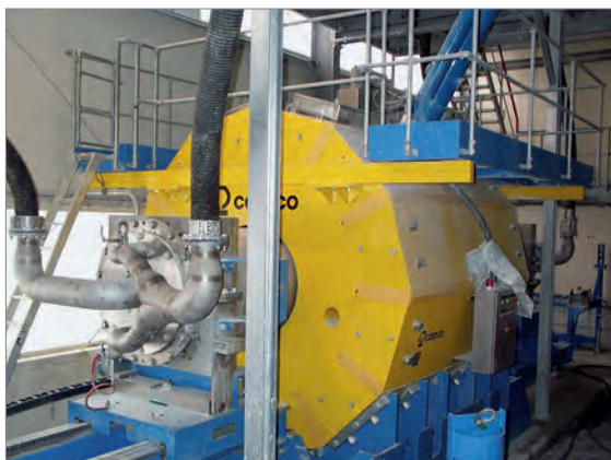
Fig. 11: High-field magnetic separator, super-cooled using liquid helium for separating ferrous minerals from kaolin, photo: Amberger Kaolinwerke Eduard Kick GmbH & Co. KG (with kind permission).
